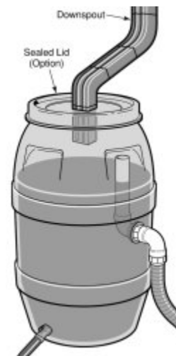
Typical Manufactured Urban Rain Barrel Design with added accessories (Source: Composters.com, A subsidiary of The Green Culture ®)
